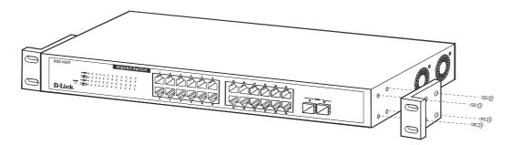
Figure 2- 2. Fasten mounting brackets to Switch
